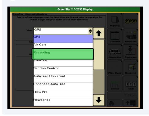
The "Recording" selection will show which element of recording is incorrect or missing
