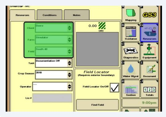
Verify the Task is set to the task the Operator is performing. Ie. Planting/Harvest/Post-Emerge Application
