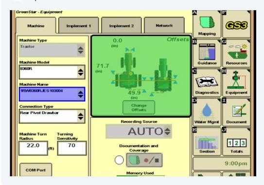
Tip! Also verify that the "Recording Source" reads "Auto" and is greyed out. This means that the display recognizes the implement that is connected.
