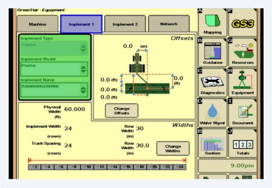
12 Verify correct width(s) and correct offset(s) are entered
